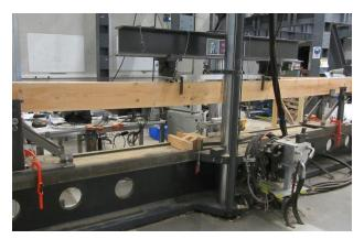
Figure 2: Destructive bending test on Douglas fir specimen at NUIG.
